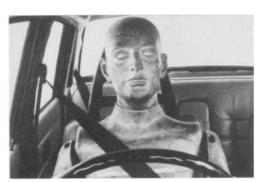
1. Sven is an electronically monitored humanoid used to evaluate passenger protection in Volvo's Safety Research Programme...
