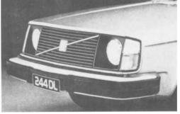
8. Energy absorbing bumpers prevent structural damage to body in `parking speed' impacts up to 5 k.p.h.
